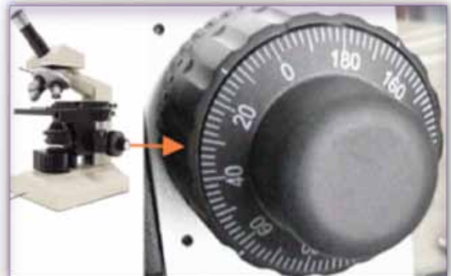
Fig. 3. The microscope's fine focus adjustment can be used to measure the distance between the lines marked on the slide and the line marked on the bottom of the coverslip.
