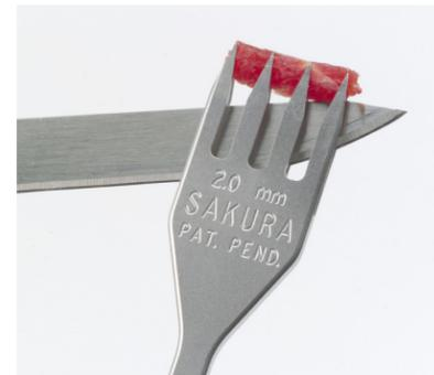
Tissue-Tek Accu-Edge Grossing Forks hold the tissue in place while sliding a trimming or scalpel blade against the outer surfaces of the fork, resulting in a section of the desired thickness between the tines.
