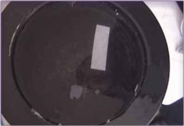
Fig. 2. Filter paper strip settles to the bottom of the water bath leaving the paraffin section floating on the surface.
