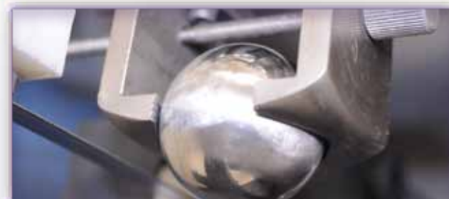
Fig. 4. Metal resurfaced femoral head loaded onto Exakt Macro Saw. Note the scuffed cap surface to facilitate firm placement in the clamp and the offset alignment.
