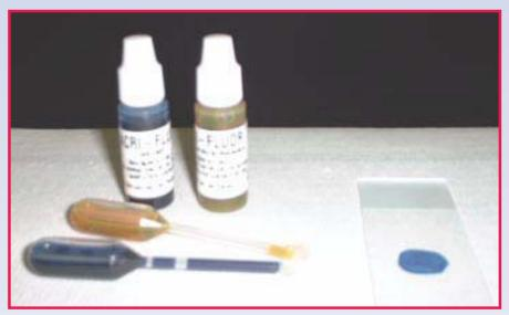
Fig. 5. Acri-Fluor Fluorescent Stain Kit<sup>™</sup> (Scientific Device Laboratory, Inc.).
