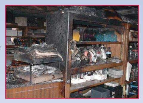
freezer leads one to believe that ignition was probably caused by the interior thermostat after the requisite accumulation of vapors. It was a big bang for such a small volume of liquid.
