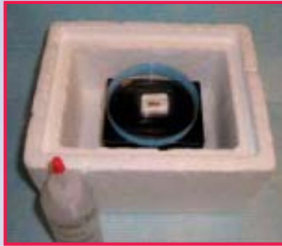
Fig. 4. Plastic Petri dish (blue) is supported by a platform to prevent tipping into the LiqN 2 inside a styrofoam box.
