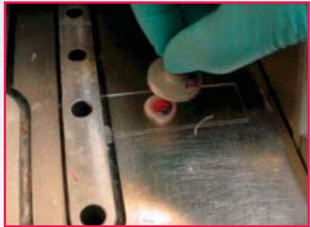
Fig. 5B. A chuck is inverted onto the tissue sample as it begins to freeze.
