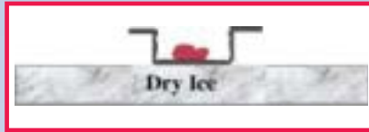
Fig. 2. A solid block of dry ice may be used to freeze tiny samples in molds containing OCT in order to obtain a totally flat block face.
