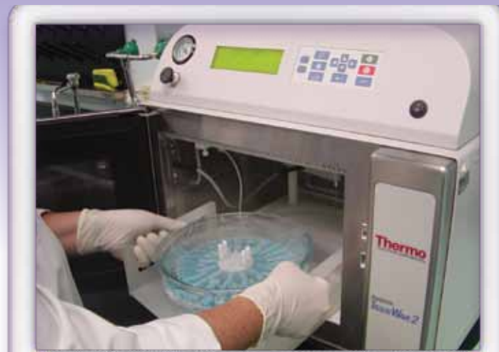
Fig. 2. Loading standard cassettes containing bones into the microwave processor.
