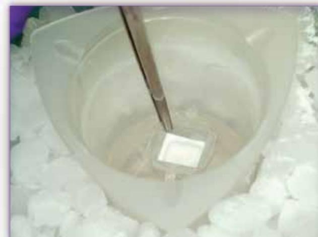
Fig. 3. Mouse brain tissue block being frozen by the forceps immersion method. In this method, only one or two blocks can be frozen in cold 2-methylbutane at a time, requiring specific hands-on time by the technologist. It also requires a large volume of cold 2-methylbutane.
