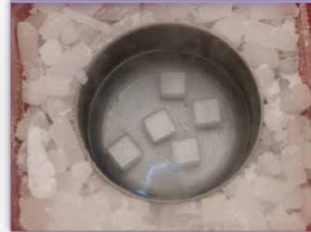
Fig. 1. Mouse brain tissue blocks being frozen by the full immersion method. The blocks are fully immersed in prechilled 2-methylbutane. The dry ice surrounding the bowl helps maintain proper freezing temperature.
