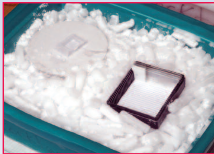
Fig. 3. Cryostat sections are placed immediately into a slide box precooled in dry ice.
